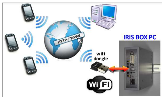
WIFI connectivity through the USB dongle.
