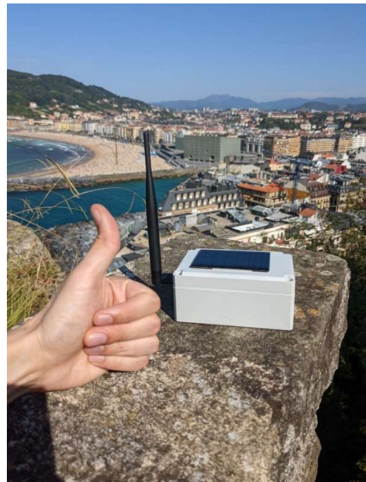
Embedded solar panel powered Isurlog LoRa outstation at the Urgull mountain in San Sebastian (Spain), linked to ISURKI's headquarters based LoRaWAN gateway through 13 km of hilly terrain. ↑ ↓
