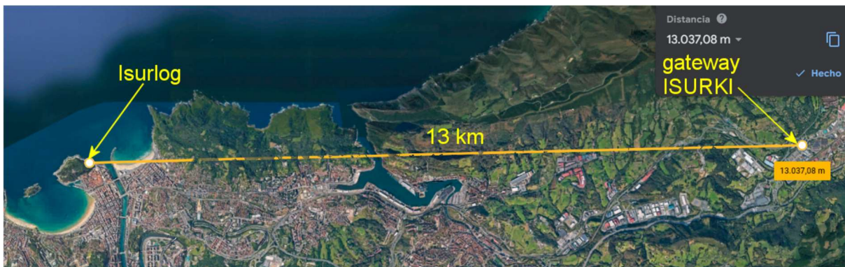
Embedded solar panel powered Isurlog LoRa outstation at the Urgull mountain in San Sebastian (Spain), linked to ISURKI's headquarters based LoRaWAN gateway through 13 km of hilly terrain. ↑ ↓
